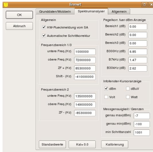
Figure 3.2: View of the Spectrum analyzer, option menu item
