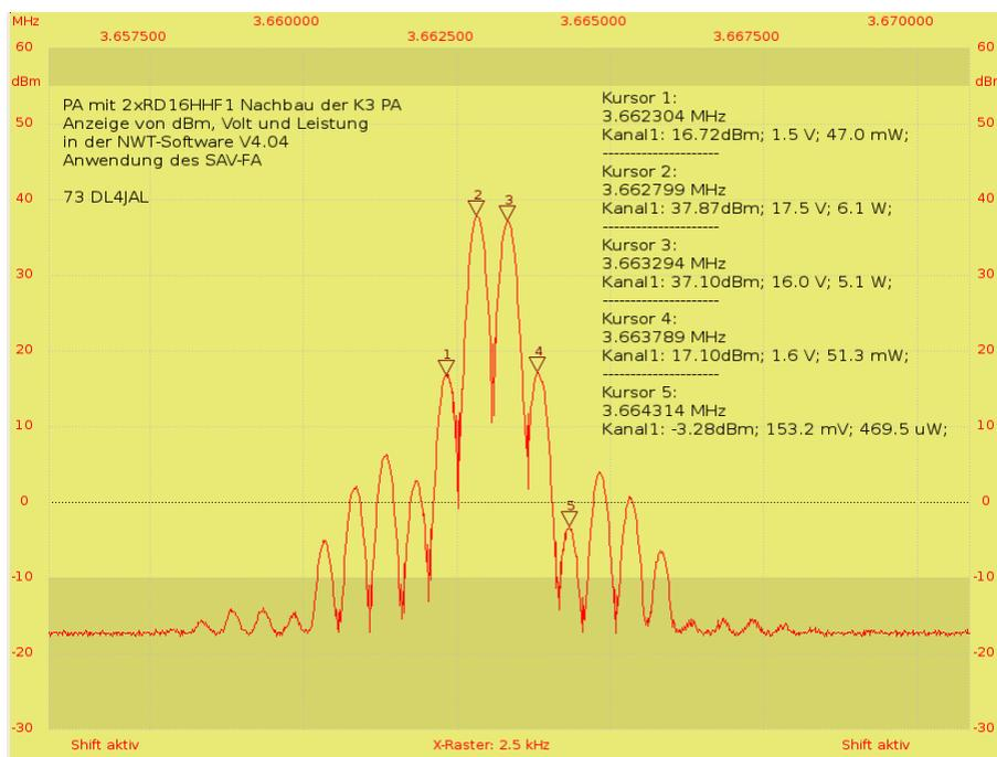
Figure 4.2: SAV view. My PA in the PicAStar, two-tone control 500Hz distance, almost full scale.
