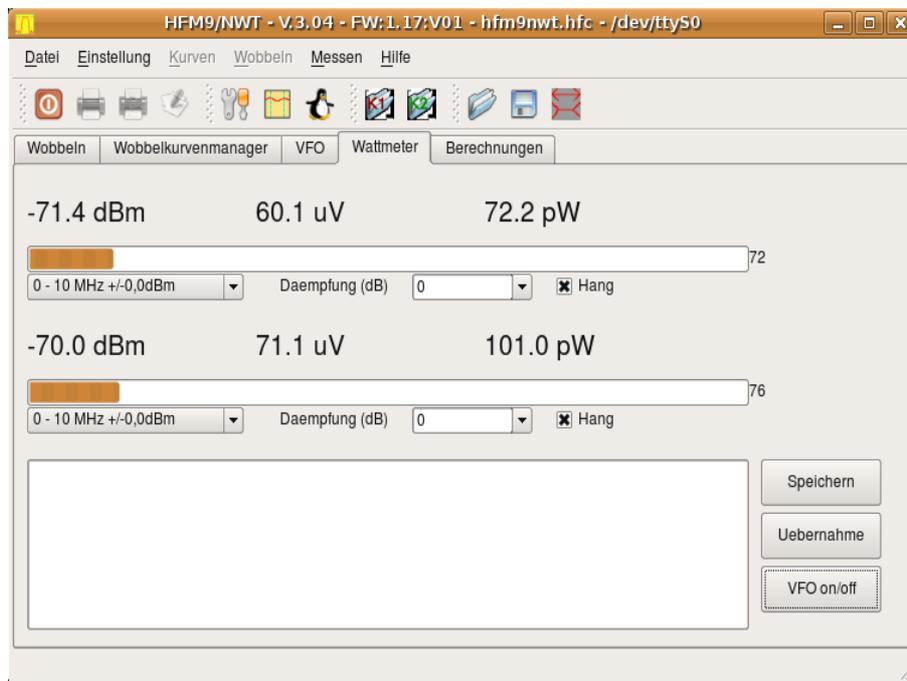
Figure 3.10: Wattmeter worksheet view without VFO
