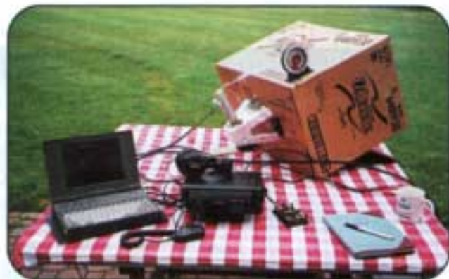
Photo F. Tony Monteiro's +20 dBi waveguide horn for 2401 MHz AO-40 satellite reception. (AA2TX photo)
