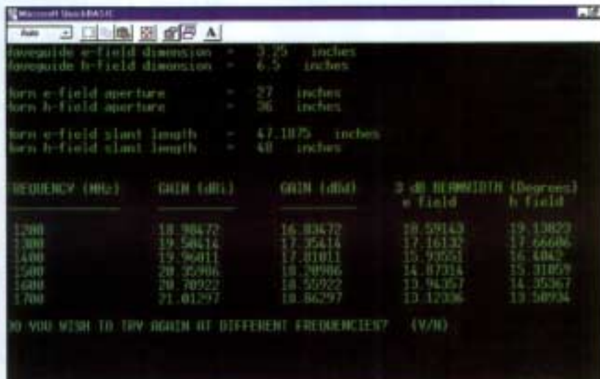
Figure 2. Gain analysis of the Ewen horn (analyzed using Horngain.xls by N6TX)
