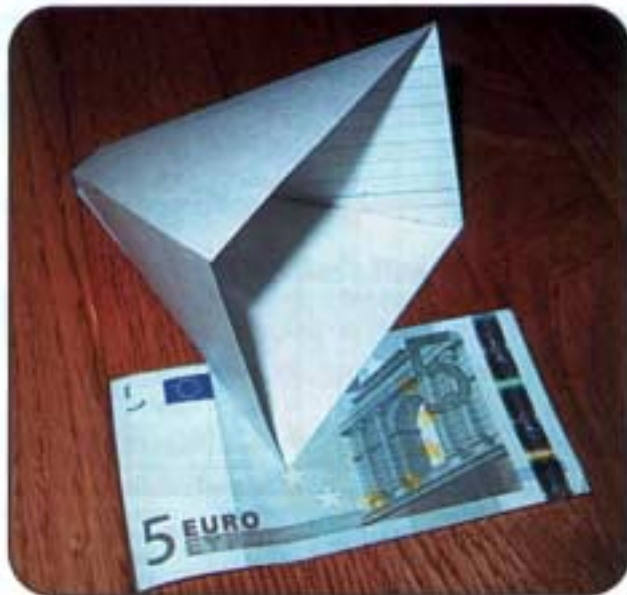
Photo G. One-twelfth scale paper mockup of the proposed SETI Horn of Plenty. (N6TX photo) →
