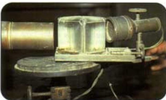
Photo D. Early Bose waveguide horn antenna. (Photo courtesy Dr. D. T. Emerson, AA7FV)
