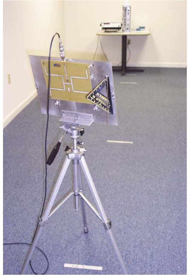
Figure 18 SARSAD far-field measurements in QorTek compact antenna range
