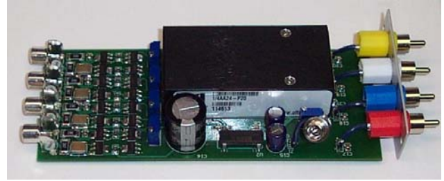
Figure 8 High-voltage driver amplifiers (circuit board)
