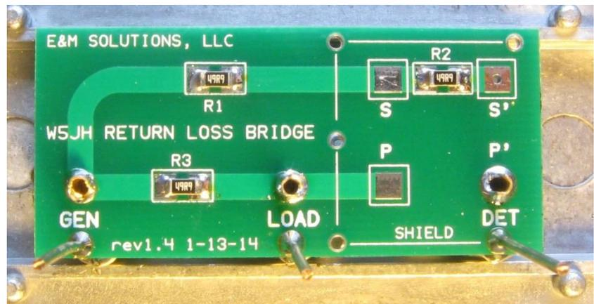
Solder all three of the 49.9 ohm, 1% resistors to the PCB. An extra resistor is supplied... just in case 😊
