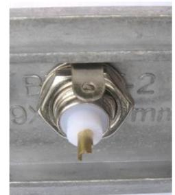
Position all three BNC connectors and their solder lugs as shown, then dry fit the PCB onto the solder posts. When you are satisfied everything fits you may tighten the nuts. It might be necessary to reposition one or two of the connectors if they shift while snugging up the nuts.
