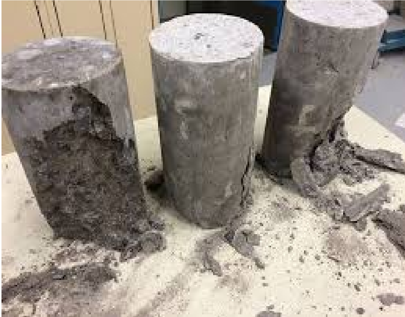
Figure 8 - Compressive strength test (a) cylindrical specimens and (b) cubic specimens
