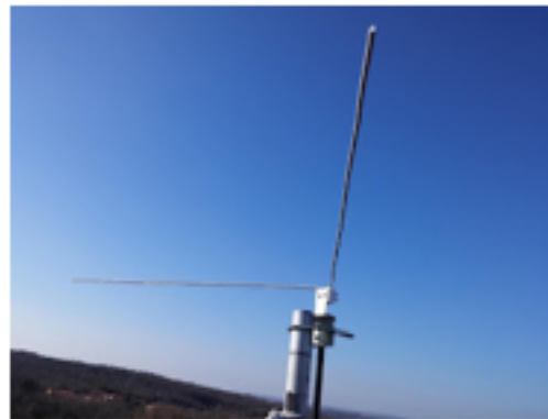
137 MHz Weather SAT V-dipole antenna
