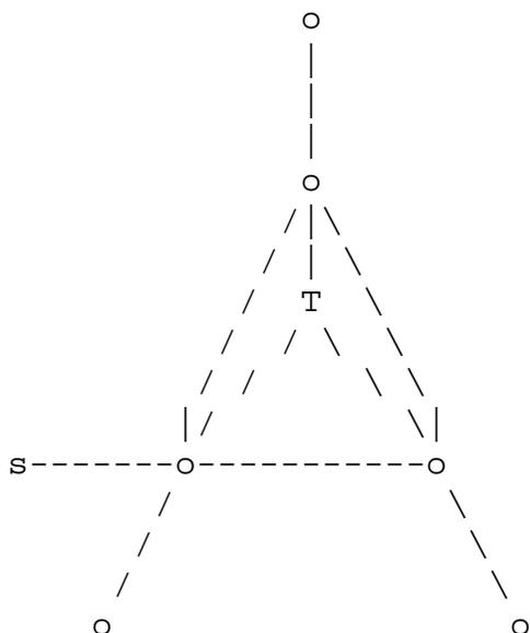
This is not quite to scale, of course. "T" is your tower base. "o" is a ground rod. The radials, tied to the tower legs, spread outward, with 8 foot deep ground rods connected every 16 feet. The first set of rods is connected together to form a triangle. There should also be a ground strap from this system to the ground system for your home (service entrance, "s").
