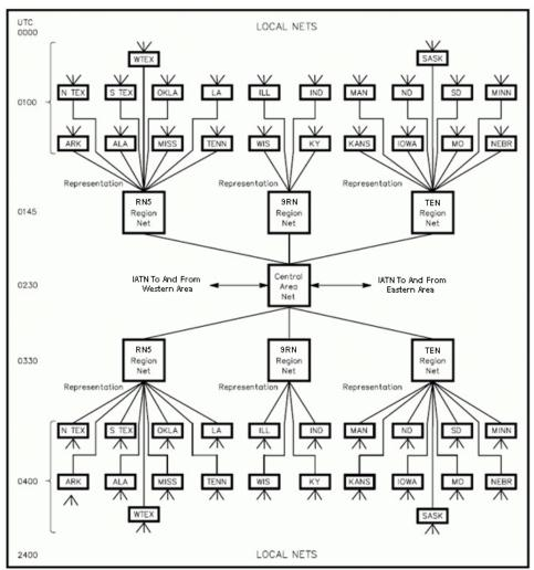
Figure 3: Example of Manual Net Structure
