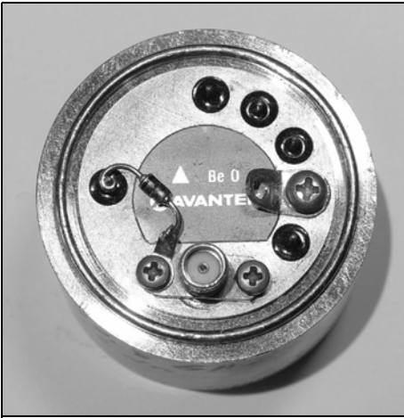
Fig 7: A YIG oscillator with no FM mode.
