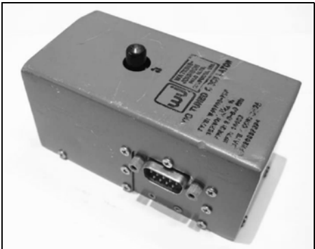
Fig 13: An example of a YIG oscillator with built in YIG driver.
