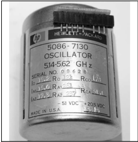
Fig 8: An example of a HP YIG oscillator with non standard operating voltages.
