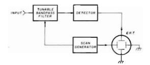
fig. 4. Tuned radio frequency (TRF) spectrum analyzer. Tuning is accomplished by adjusting the bandpass-filter frequency.
