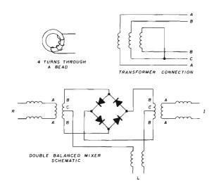
fig. 15. Construction details for winding transformers and baluns used in the r-f section.
