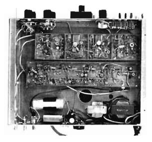
Bottom view of spectrum analyzer chassis showing the lassembly (along front of chassis, top) and logarithmic amplifier (center). Power supply components are located along the rear of the chossis, bottom.
