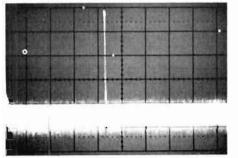
fig. 27. 1-1 gain adjustment. BW 250 kHz, Scan 10 MHz/division, Generator frequency 40 MHz; generator output about 4 divisions. The 1-1 gain is set too high, which snifts the baseline up two divisions. This results in a loss of about 20 dB of dynamic range.
