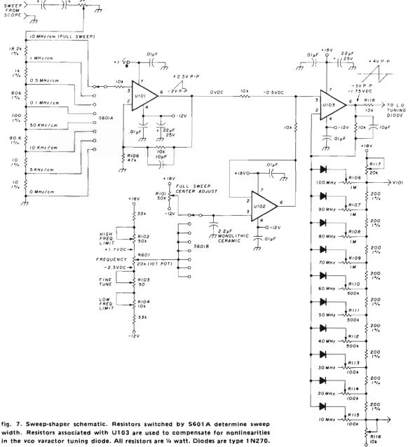
in the vco varactor tuning diode. All resistors are 1/4 watt. Diodes are type 1N270. ICs are uA741.
