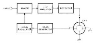
fig. 5. Simplified block diagram of a superheterodyne spectrum analyzer, Local oscillator is suned by the scan generator.
