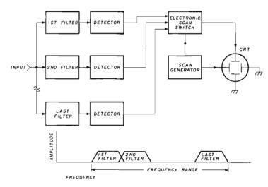
fig. 3. A real-time spectrum analyzer. Filters are spaced to provide continuous coverage of the frequency spectrum.
