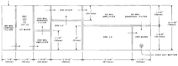
fig. 14. Rf-section dimensions.
