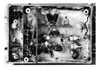
Clossup view of the voltage-controlled oscillator. Main circuit is in the compariment to the right; connectors for output to the first mixer and tracking generator are in compartment on 18/1.
