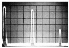
fig. 23. Second harmonic of transmitter operating at about 4 MHz. Second harmonic is down only about 32 dB.
