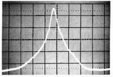
fig. 18. 10-kHz bandwidth position after alignment. Horizontal scalo: 10 kHz per division.
