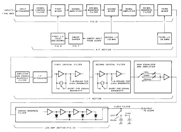
fig. 6. Complete superheterodyne spectrum analyzer described here. Each block represents an individually shielded section or assembly.
