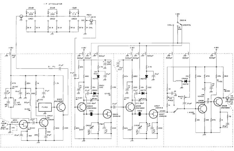
fig. 11. I-f section schematic. All resistors in the attenuator must be 1% tolerance. Resistors must be added in series or parallel to obtain 51 ohms ±1% with R601. Feedthrough caps are 500 pF.
