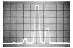
tig. 26. Output of a commercially made ssb transmitter into a 50-ohm load with carrier inserted at about 3.8 MHz. Scan 500 kHz/division. Note spurious signals at about 3050 kHz and 4550 kHz.
