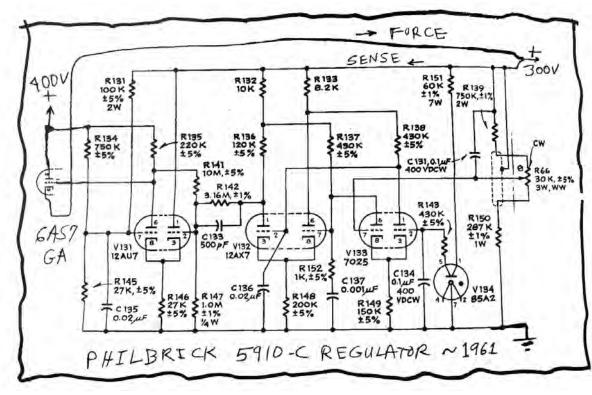
high-line. Also, it has submillivolt gain error, for line, load, or ripple.
