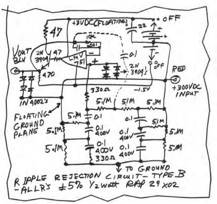
ripple-rejection, using my NoiseMaker (schematic is on my Web site) to try to cut the ripple of an 85-mV p-p (26-mV rms) noise at a 26-kHz nominal switching frequency, with lots of harmonics at 52 and 78 kHz. Although the Type A circuit improved the 26 mV to 0.88 mV, Type B did a bit better at 0.83 mV. But that was NOT unexpected. So it's not too hard to get a 30-dB noise improvement by employing a cheap, low-noise op amp, such as LMV751.
