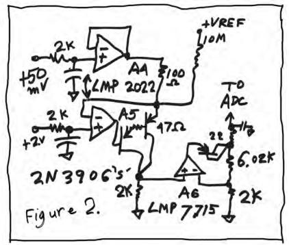
resistors, the common-mode rejection ratio (CMRR) of the third amplifier can be as poor as 37 dB with respect to the input or 31 dB at the output. They said they were assuming there would not be much CM noise.
