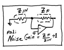
the noise gain is not at least 10 (or as stated). But, refer to NSC's App Note LB-42. Reactances: If we add a feedback capacitor across RF, the noise gain can be high at low frequencies, but
