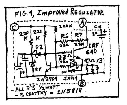
voltage across R5 to decrease. So in case of a short, or a very heavy load, the current limit folds back, and the heat in the FET decreases. That sounds pretty good. But what if you need to start-up a heavy load? That current through R6 would prevent the limiter from starting in case of filament inrush current, or filter capacitors that need to be charged.
