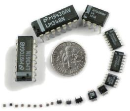
1. The electronics industry has evolved as packages have gotten smaller and smaller. For example, the 14-pin dual-inline package (DIP) is now today's micro-SMD.
