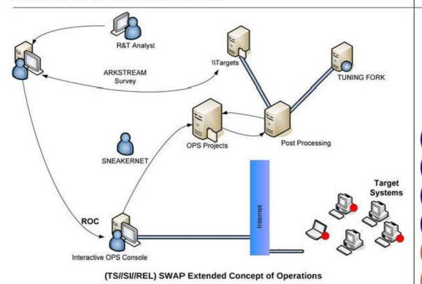
(TS//SI//REL) This technique supports single or multi-processor systems running Windows, Linux, FreeBSD, or Solaris with the following file systems: FAT32, NTFS, EXT2, EXT3, or UFS 1.0.
