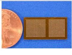
(TS//SI//REL) TRINITY uses the TAO standard implant architecture. The architecture provides a robust, reconfigurable, standard digital platform resulting in a dramatic performance improvement over the obsolete HC12 microcontroller based designs. A development Printed Circuit Board (PCB) using packaged parts has been developed and is available as the standard platform. The TRINITY Multi-Chip-Module (MCM) contains an ARM9 microcontroller, FPGA, Flash and SDRAM memories.
