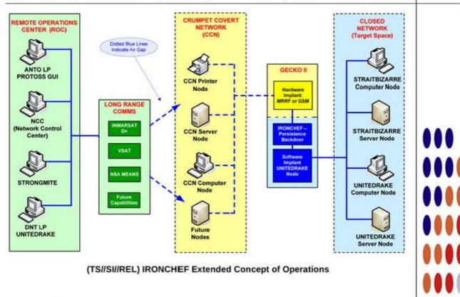
(TS//SI/REL) This technique supports the HP Proliant 380DL G5 server, onto which a hardware implant has been installed that communicates over the I<sup>2</sup>C Interface (WAGONBED).
