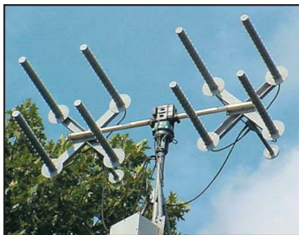
Dual quad-helix arrays for 1296 MHz, one right-hand and the other left-hand circularly polarized, are part of The SETI League's W2ETI Moonbounce Calibration Beacon.
