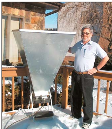
The SETI Horn of Plenty, a waveguide horn antenna for 1.3 to 1.7 GHz designed by the author, has been duplicated by dozens of SETI League members around the world, for classroom demonstrations as well as observational radio astronomy and SETI.
