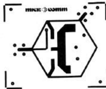
Fig. 4. Typical microstripline artwork.
