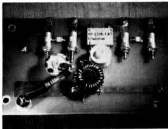
Double-balanced mixer layout for 1296 MHz, showing component placement on the printed-circuit board (see fig. 3).
