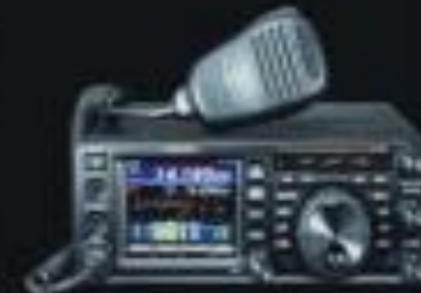
CW/SSB/AM/FM/C4FM 144/30/344/430 MHz Wide-Coverage 100 W All Mode Transceiver (244/430 MHz 50 W) FT-991A (Real-Time Spectrum Scope included)
