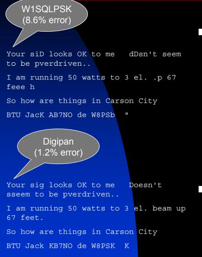
Processing incoming audio is CPU intensive! If you see strong waterfall signals, but poor copy, terminate other programs that might be running on your computer and stealing CPU cycles!
