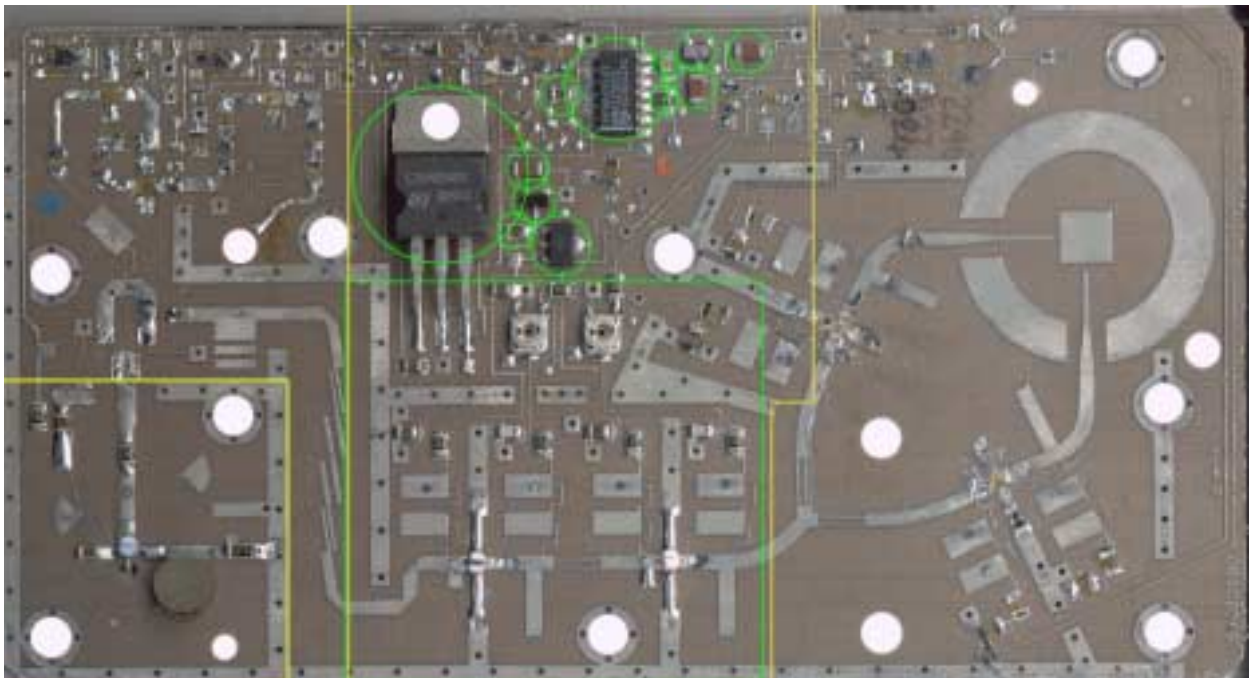
Figure 2 - Remove, but retain, all SM components outside of Green borders - Cut board on Yellow borders.
