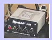
The Signalink USB Sound Card has the advantage of it's own independent sound card, and <u>volume controls on the device</u>. Only requires two cables (provided), one for the connection to your radio and the other (USB) to connect to your computer.
