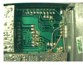
The picture to the left shows the inside of a KF161 from a different production batch. If you have a KF161 like this, then you need to repair 3 PCB traces.
