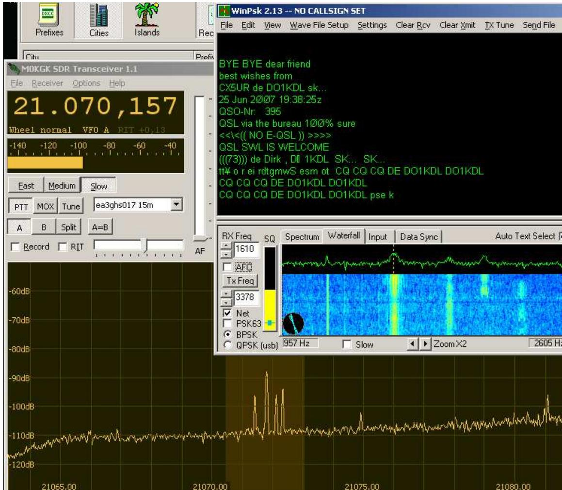
test 1 Connect the antenna to the receiver, read the noise floor level. Disconnect the antenna and read the noise level again. If the level is the same (here is the same) the total receiver gain is not sufficient. The noise that you view in the screen is internal receiver noise, not atmospheric noise.
