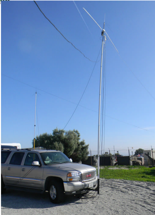
5-section, 20' heavy-duty aluminum flagpole from Harbor Freight with 4' wooden pole attached to top section
