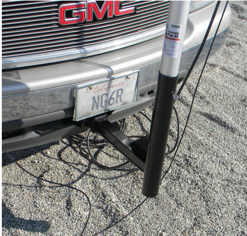
Hitch mounted flagpole holder from Amazon.com; ancillary front trailer hitch had previously been installed on vehicle
