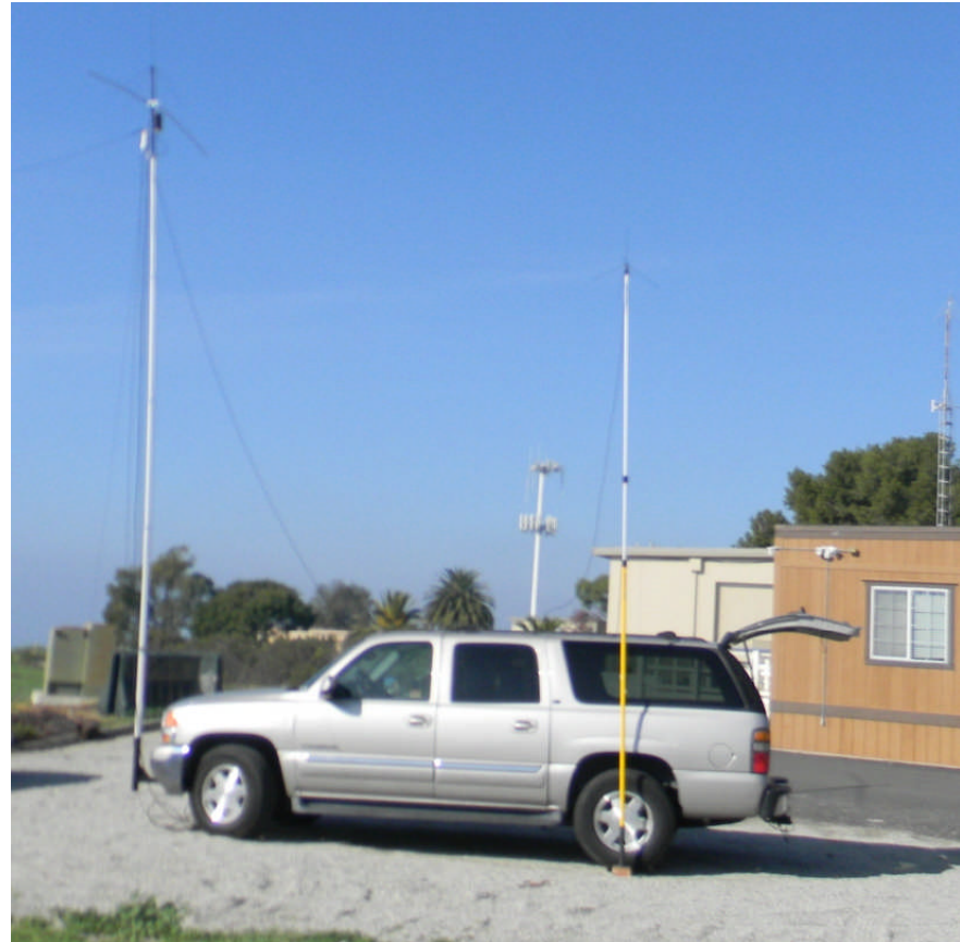
3-section, 23' extension pole from Lowe's (right in photo), only partially extended here
