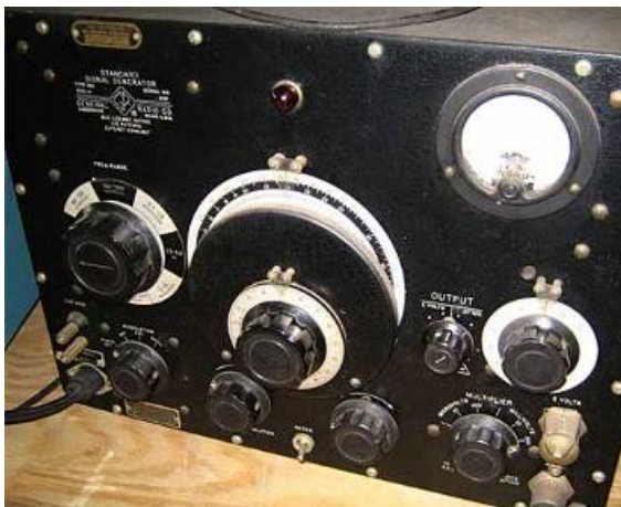
Figure 6: General Radio Standard 1001A signal generator
