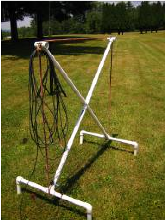
Figure 12: SuperSID loop similar to ours. Photo taken at Green Bank 2010
