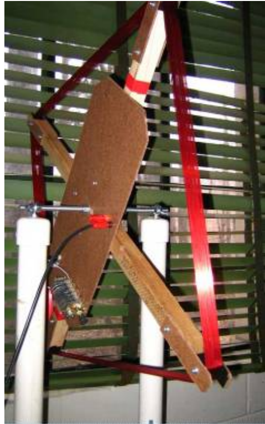
Figure 5: Our loop: Primary = 120 turns of #30 wire. Secondary = 12 turns of #30 wire. Tuned by 500 pF tuning condenser. Frame approximately 19" square
