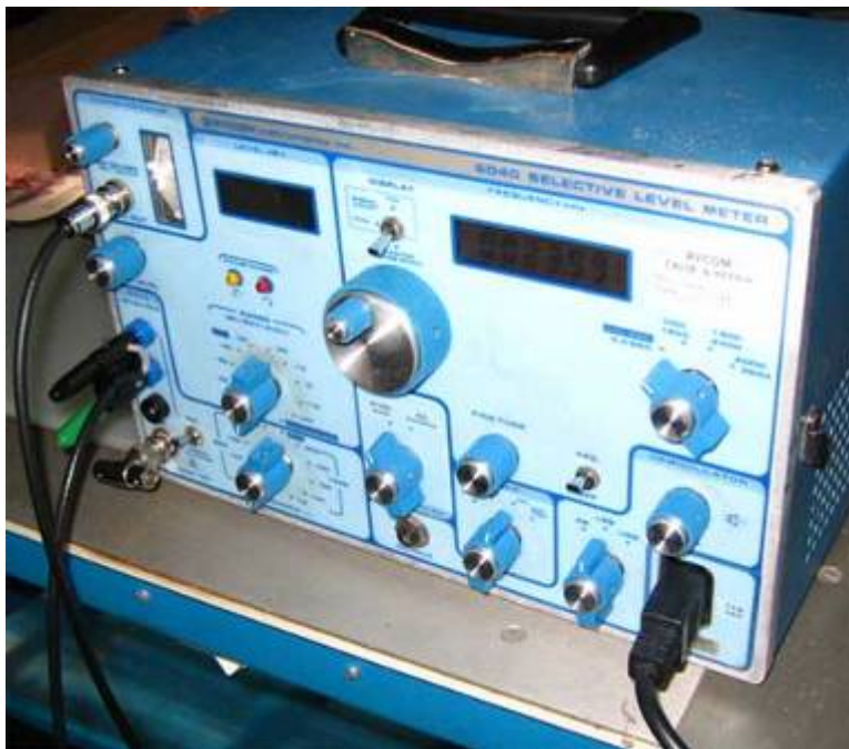
Figure 7: Rycom 6040 selective level voltmeter
