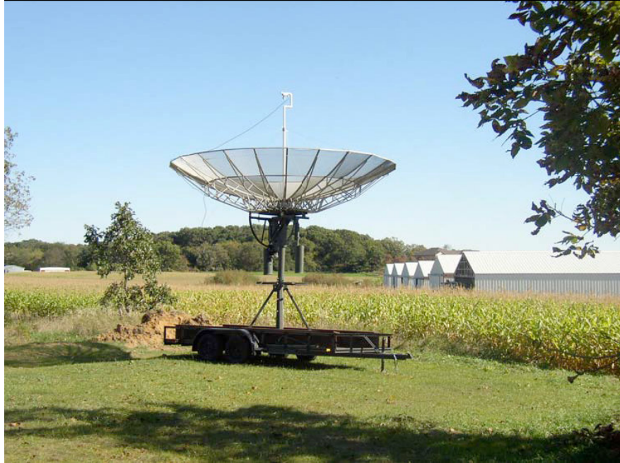
Figure 14: The 16-foot dish (the 12 GHz feed horn shown has been replaced with a 1420 MHz feed horn/LNA assembly)
