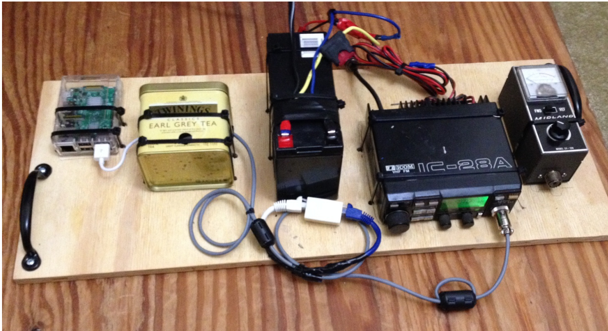
Prototype Deployable Digital Relay Station -- home made "$10TNC" soundcard-based interface Antenna coax wiring is not yet installed. Battery charger isn't shown.
