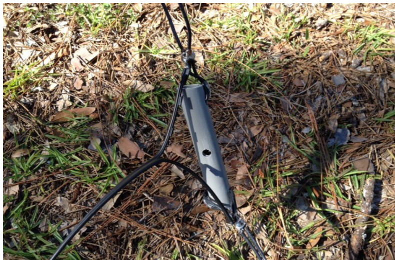
Figure 7. View of the center insulator. Wires are soldered. For long term use, the balanced line would be wrapped \frac{3}{4} around the center insulator as a stress relief and held in place with a non conductive fastener such as nylon rope or sunlight resistant zip-tie.
