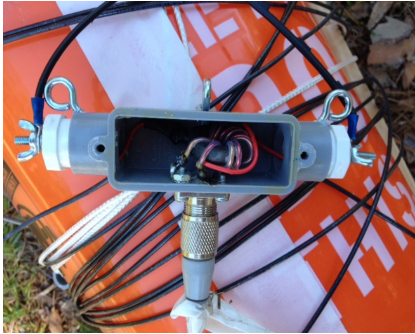
Figure 6. Inside view of the balun, including the toroidal 4:1 transformer
