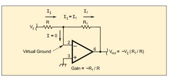
Figure 3—The inverting amplifier.
