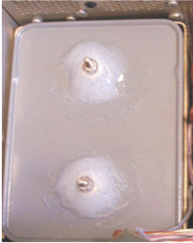
(HV filter capacitor)
