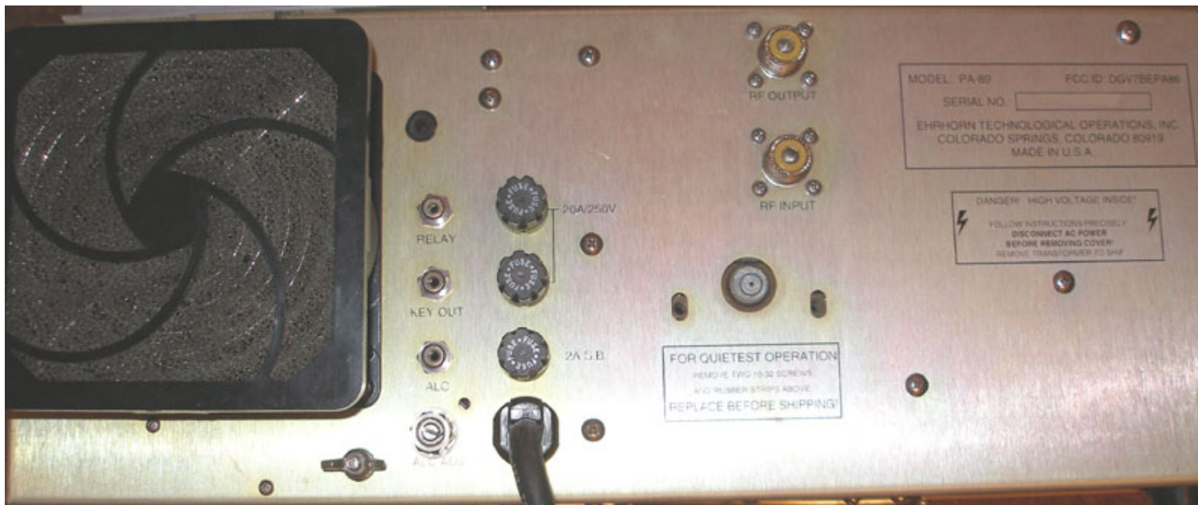
Above is a photo of the rear panel, showing the factory installed auxiliary cooling fan and washable air filter. The "key out" port is for QSK operation only, it insured proper key sequencing, and need not be used when PTT SSB is used.
