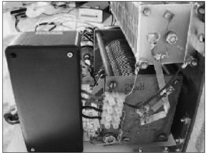
Figure 12 — Detailed view of the interconnection of the tuning elements.
