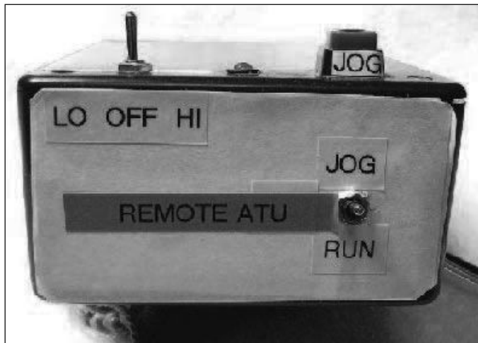
Figure 7 — The simple in-shack motor control box.
