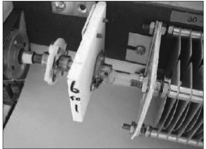
Figure 4 — A 6:1 vernier reduction drive makes the capacitor turn slower but still faster than the coil. The rotating capacitor applies all values from 30 to 300 pF while the coil rotates less than 90°.
