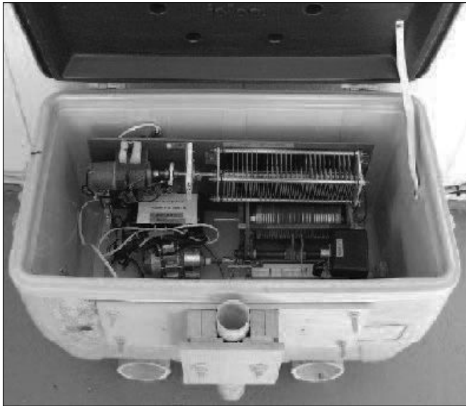
Figure 3 — A picnic cooler provides an outdoor moisture resistant enclosure.
