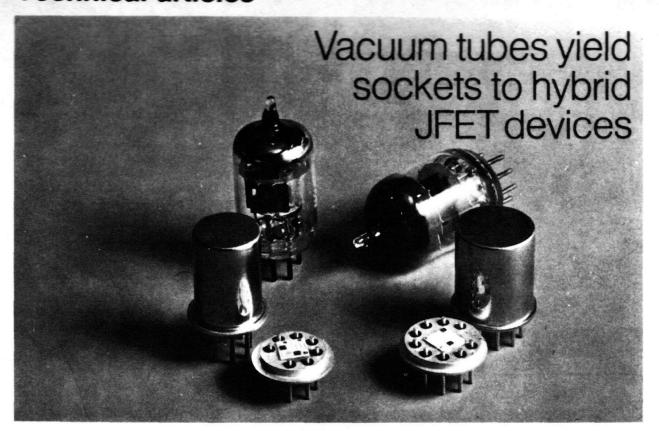
Thanks to high-voltage JFET technology, hybrid circuits called Fetrons exhibit virtually no aging, and also offer higher gain than do their vacuum tube counterparts
