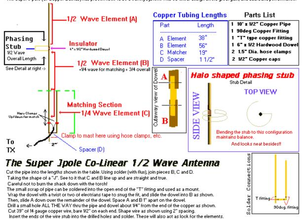
Solder the two Caps on the open ends to keep water out. Attach the two hose clamps approx. 2" up from bottom. Clamp the bare ends of the coax to the elements with these clamps. To tune, slide feed up and down for match!
