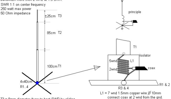
T3 = 8mm diameter (tune to best SWR by sliding it in or out of T2).
