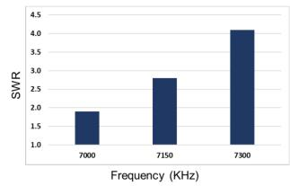
2) The values for SWR *decrease* on all measurements of the lowest, middle, and highest frequencies. In this case, the resonant frequency is too high, which means the antenna is too short.
