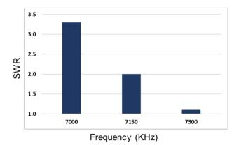
3) The SWR value for the middle frequency is lower than the SWR values for the lowest and highest frequencies. In this case, the resonant frequency is inside your band. If the SWR value for the lowest frequency is lower than the one for the highest frequency, then the antenna is slightly too long. Conversely, if the SWR value for the highest frequency is lower than the one for the lowest frequency, then the antenna is slightly too short.
