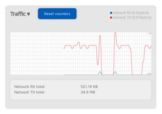
The **traffic graph** can be shown by clicking on the arrow at the top of the Traffic section. Values displayed are rough estimates, and are based on the currently active connector's traffic.
