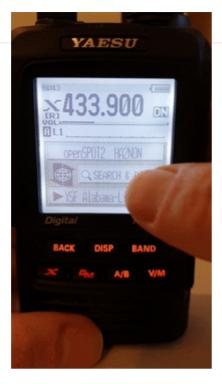
The first 5 entries will be your openSPOT4's configuration profiles. The list will contain the servers of the currently active connector. In case the currently active connector does not have a server list (ex. the Null connector), YSFReflector servers will be listed. To switch to an entry, select it using the dial and press PTT for a short time (or just tap on it in case you have a touch display).
