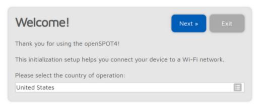
If the initialization setup won't open automatically, then you can open it by entering <a href="http://192.168.99.1/">http://192.168.99.1/</a> into the web browser while your browser device is connected to the Wi-Fi network **openSPOT4 AP**. Note that this IP address only works while the openSPOT4 is in AP mode (indicated by white Status LED), and your browser device is connected to the **openSPOT4 AP** Wi-Fi network.
