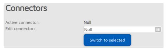
In openSPOT4 terms, a connector is the **protocol** which you use to connect the openSPOT4 to a server.
