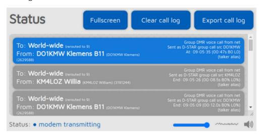
The call log displays all calls coming from the network, from the modem, or from the openSPOT4 itself (voice announcements). In modes where IDs are used as destination and source IDs (ex. DMR, NXDN®) the IDs are matched to the ID database and replaced with callsigns. You can get more information about an ID or callsign if you hover the mouse over it.
