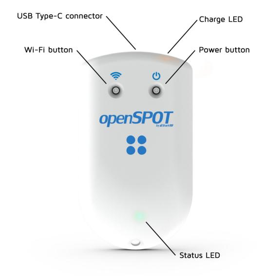
If the device is running with the factory default configuration, then there's an initialization running for about 5 seconds and the Status LED is flashing white:
