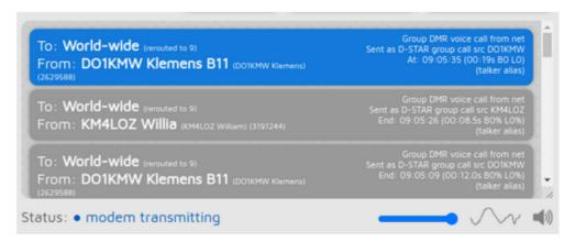
You can toggle call audio playback by clicking on the speaker icon under the call log, or with the keyboard shortcut Ctrl+M. There's a small oscilloscope view which shows call audio being played. Note that the oscilloscope view's signal levels does not actually represent the volume of the played back audio, as the openSPOT4 uses audio dynamic range compression. You can change the audio volume with the slider, or with the keyboard shortcuts Ctrl+V and Ctrl+B.
