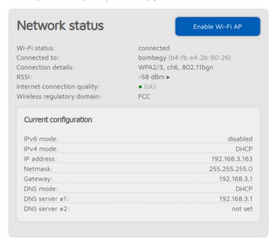
The **Network status** section shows current network status. The **Wi-Fi RSSI graph** can be shown by clicking on the little arrow next to the RSSI value. The **Internet connection quality** is determined by the openSPOT4 by periodically measuring the network latency. You can get the measured latency value by hovering the mouse above (or clicking on) the quality display circle. The **Wireless regulatory domain** is determined by the country of operation.
