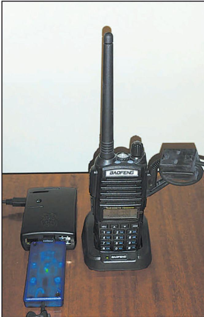
Photo A. A very compact Allstar node. The blue box is the ARS USB radio interface. Note the snap-on ferrites that I added at each end of the microphone cable.
