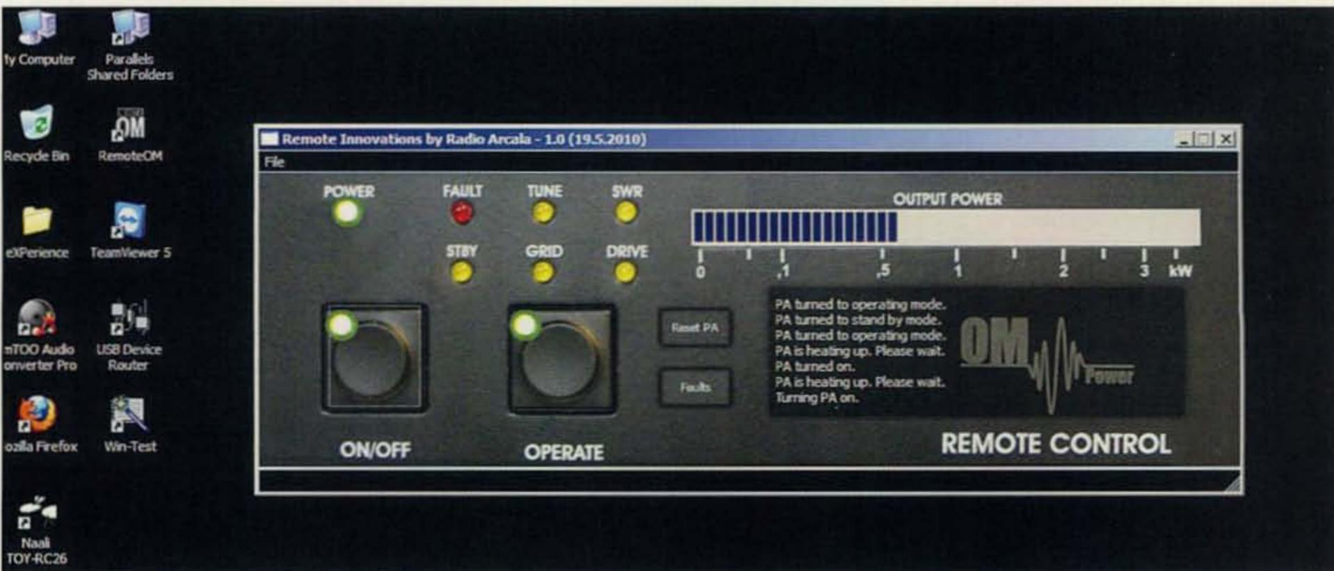
This is how the remote amplifier appears on a local computer screen. With HTTP technology, you can control each function with your mouse, see the actual power and monitoring LEDs, plus receive a stream of messages on amplifier functionality. You need not worry about the amplifier being away where it will not cause noise or interference.
