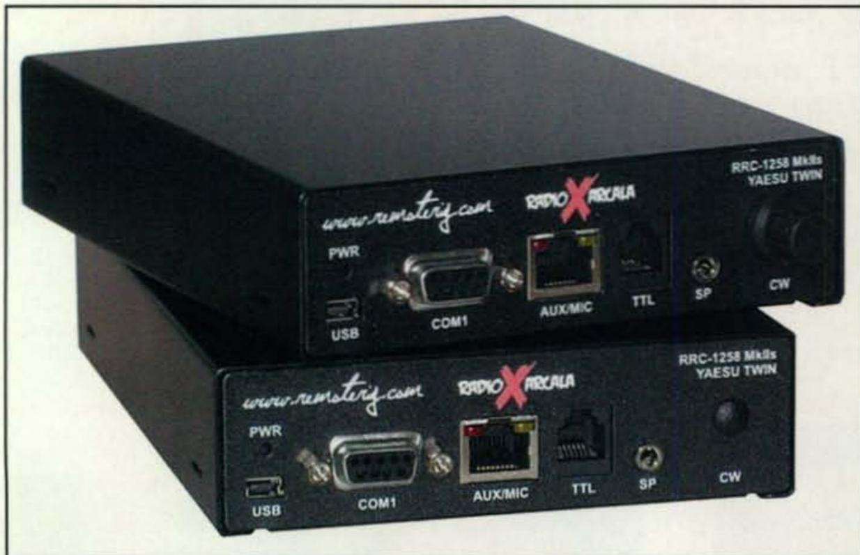
Control and remote RRC units utilize three communication channels; a simple text-based SIP protocol is utilized for radio-to-radio communication, while a UDP datagram protocol is used for control and audio streams. The RRC unit also provides two additional serial ports for connecting devices such as an amplifier and a rotator control.
