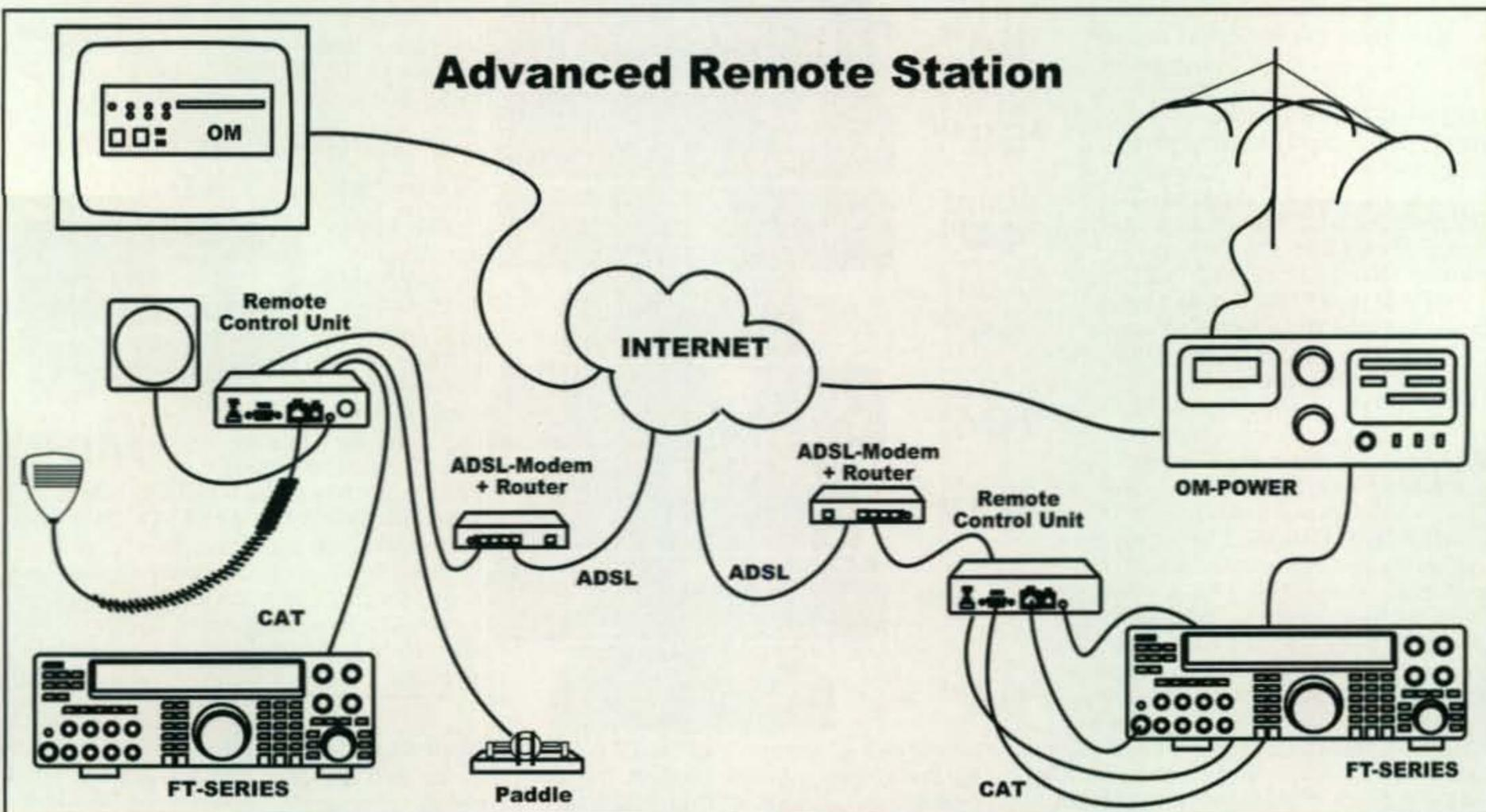
The overall station layout connects all necessary building blocks together in a simple way that today's ham operators are bound to know in the contemporary internet-dominated world. Changing between local operation and remote operation is as easy as changing the microphone and headphones. No RF or data-related cables need to be touched.
