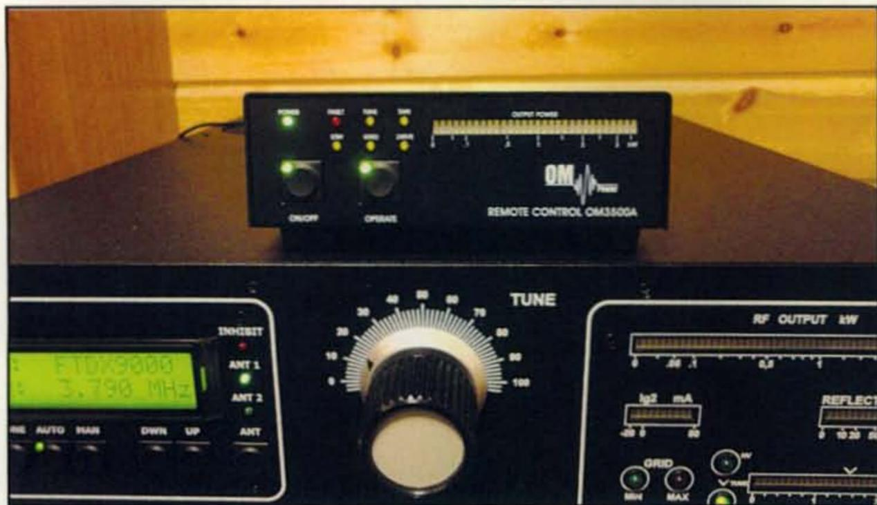
If amplifier noise and heat bother members of the household in a local operation, the small remote unit is all that is needed at the traditional station. The amplifier itself can be placed some 10 meters (30 feet) away from the station, connected over the internet.
