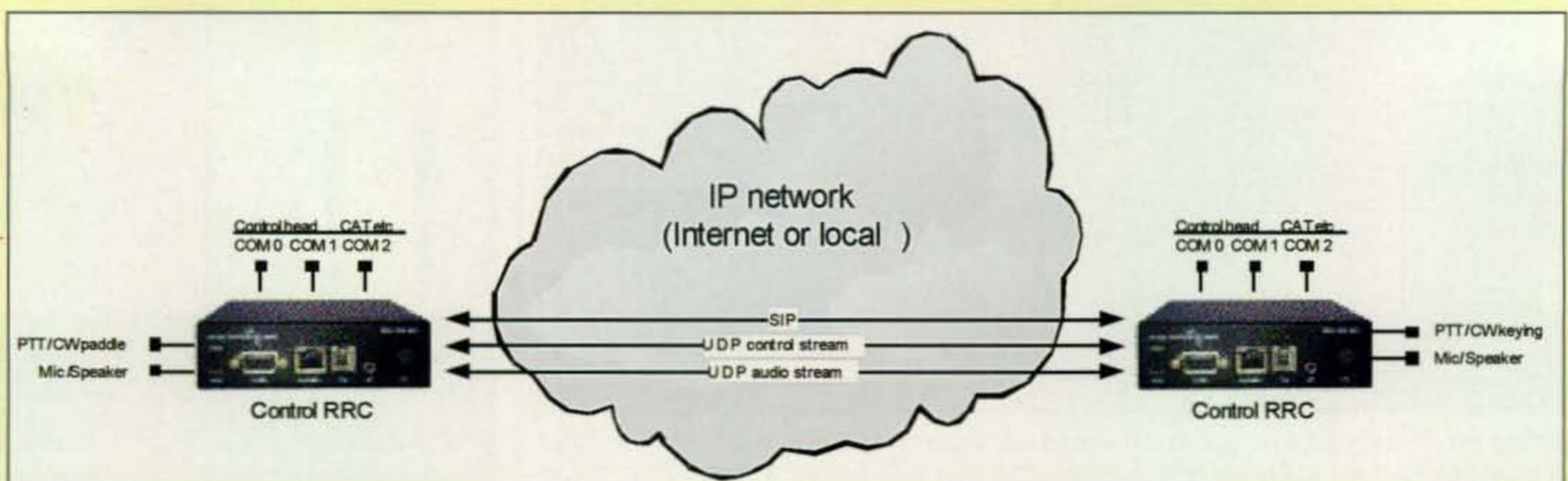
Connections and data paths between the Remote Radio Controllers at the control end and the remote end of the circuit. The two ends may be located anywhere that a broadband internet connection is available.
