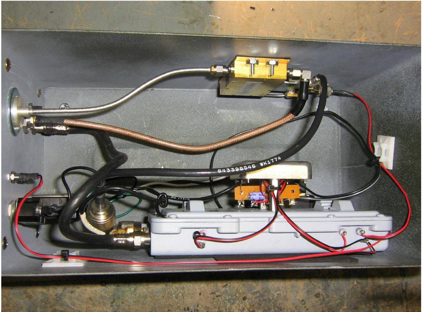
Overview of the front-panel and 1.25 GHz oscillator to HMC444 board connections.
