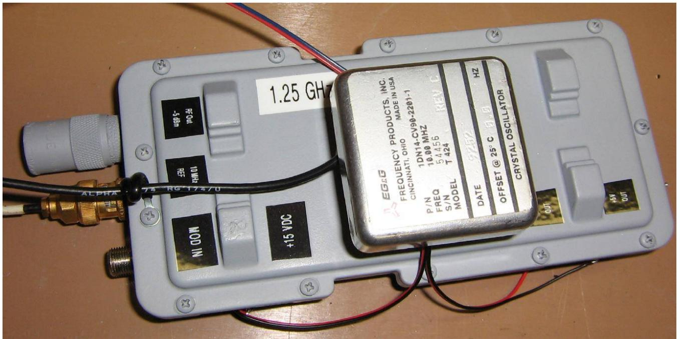
Attaching the external 10 MHz TXCO crystal to the outside of the MMDS downconverter case housing the oscillator board.
