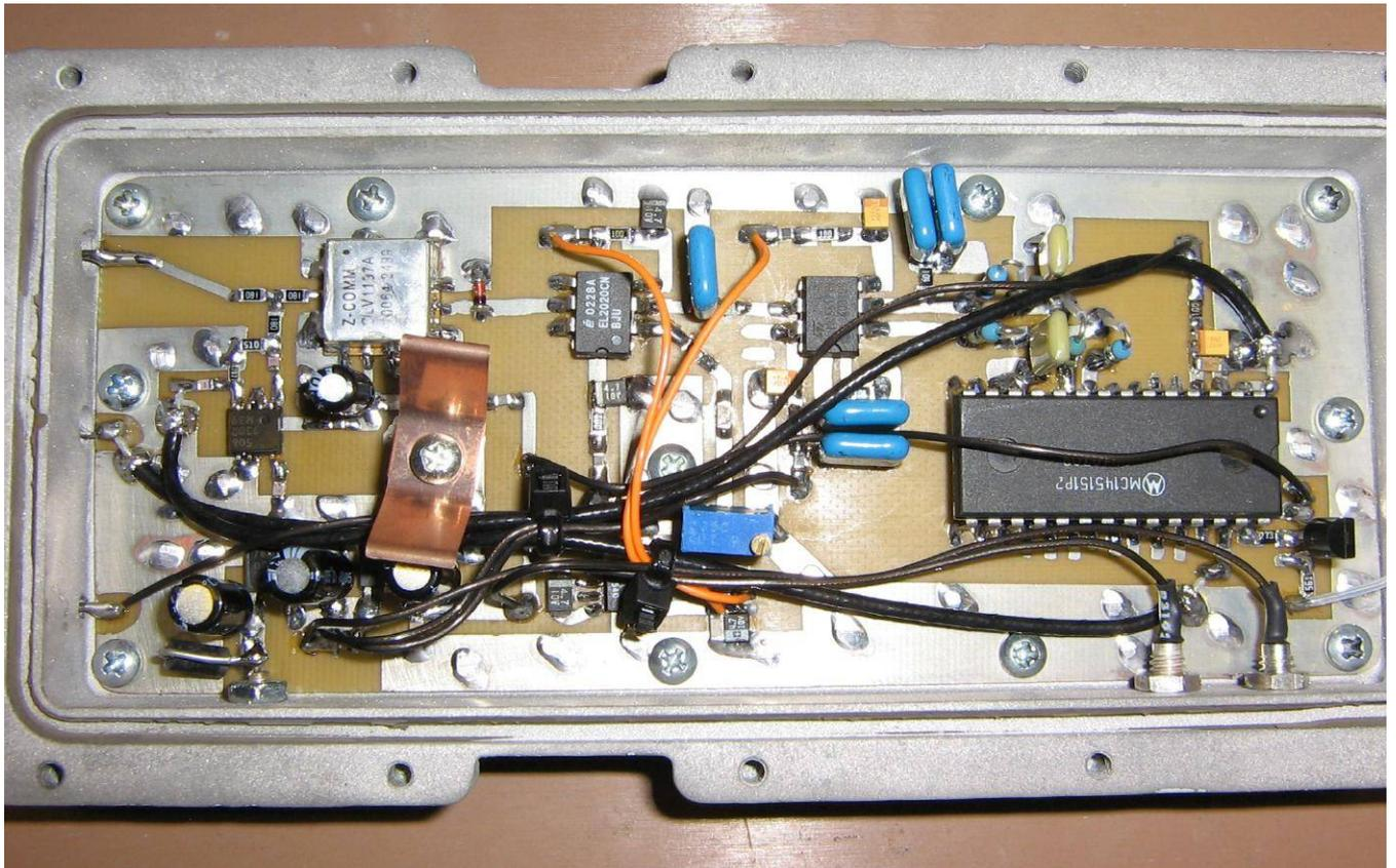
Overview of the completed 1.25 GHz phase-locked loop oscillator board.
