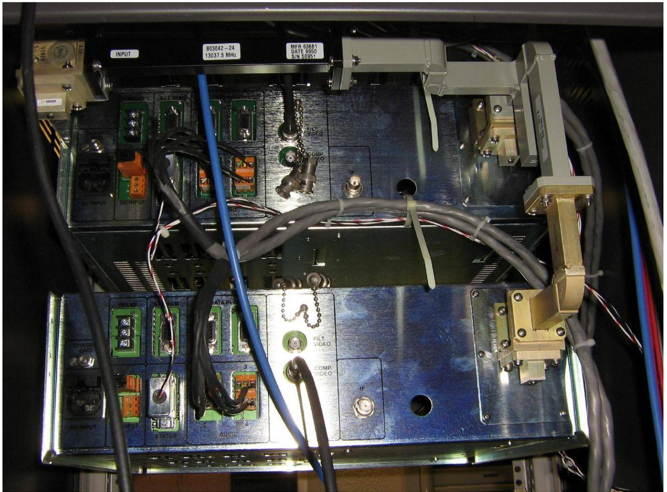
13.0375 GHz Ku-band point-to-point relay link transmitter for a local TV station.
