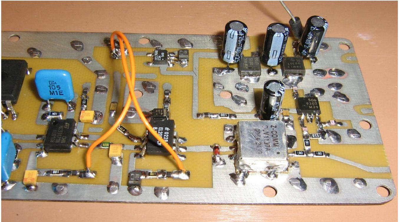
Constructing the 1.25 GHz phase-locked loop oscillator board.
