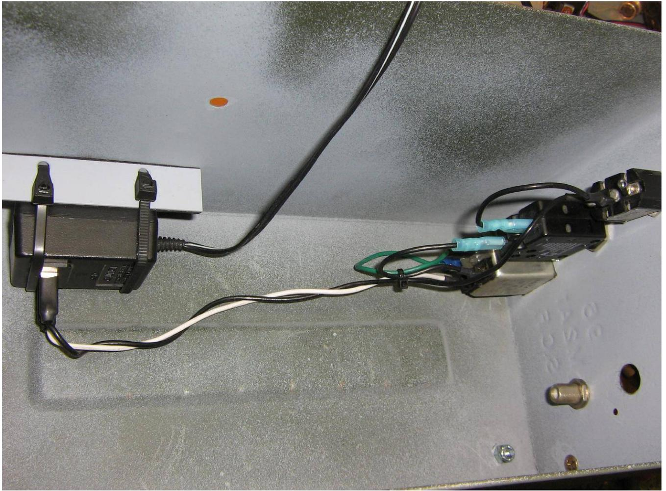
AC power input for the ammo box case we'll be using.
