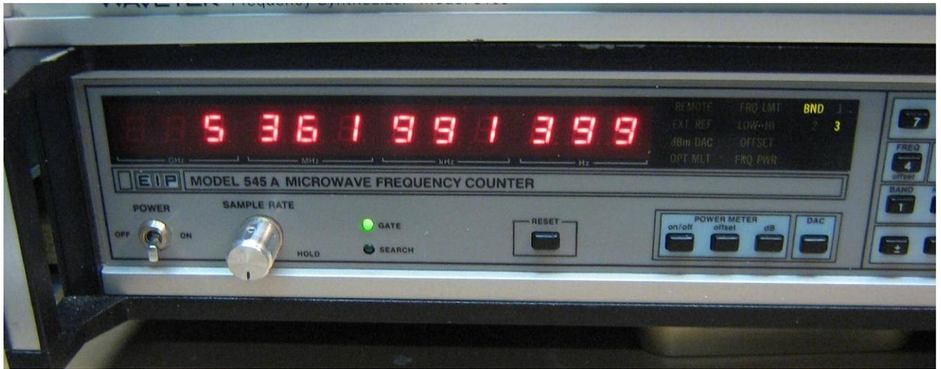
Tweaking the oscillator's final output frequency down to 5362.0 MHz, or as close as possible.
