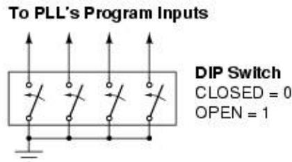
Here is an example of using DIP switches, or even regular SPST switches, to load the divide-by-ratio programming inputs on the MC145152.
