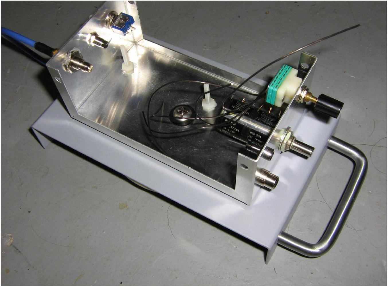
Case overview used to hold the modified VR36A receiver.
