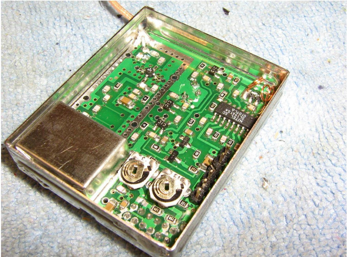
Alternate internal view of the 2.4 GHz video receiver module.
