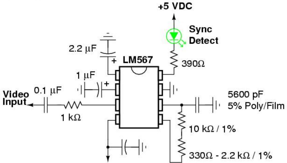
Choose value so the frequency at pin 5 of the LM567 is around 15.75 kHz.
