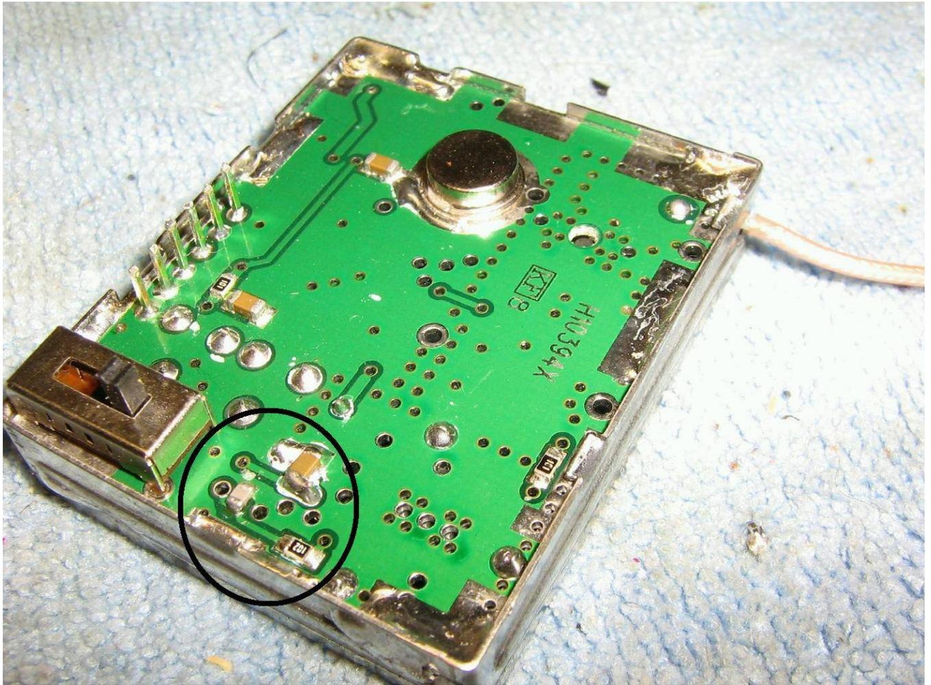
Bottom view of the 2.4 GHz video receiver module.
