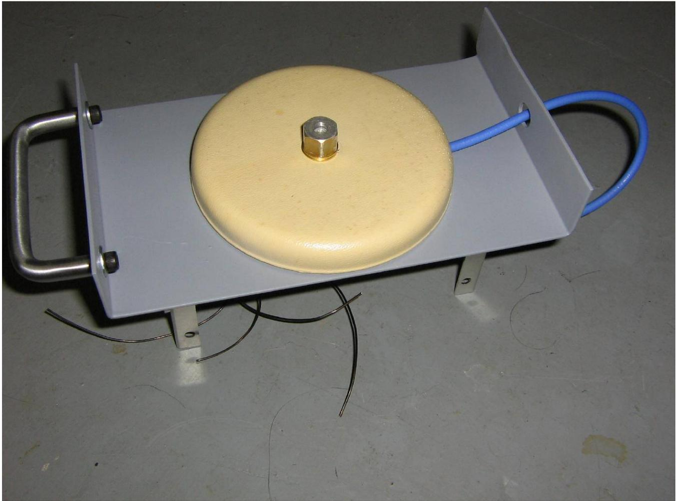
For this project, we'll mount the 2.4 GHz video receiver to the back of an old California Amplifier 2.5 GHz MMDS integrated downconverter and 22-element Yagi antenna.
