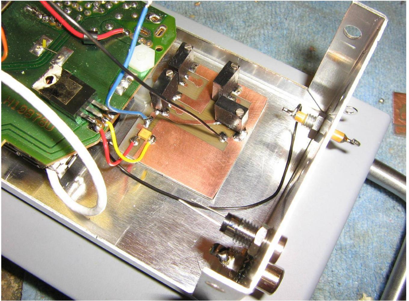
Overview of the potentiometers for setting the voltage levels which correspond to each of the four stock channels.
