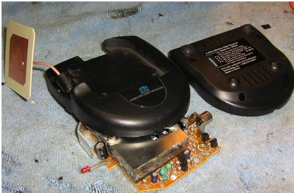
Overview of the "X10 Model No. VR36A 2.4 GHz Wireless Video Receiver" for use with X10's wireless camera systems operating in the unlicensed 2.4 GHz band.
