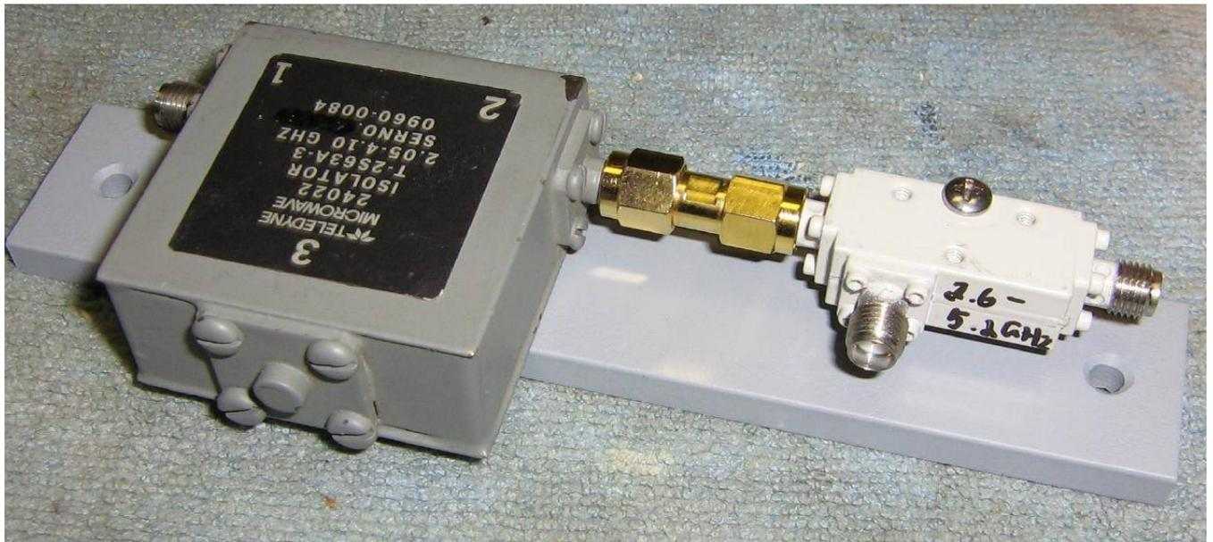
An optional ferrite isolator and a 20 dB directional coupler are added to RF output of the amplifier.
