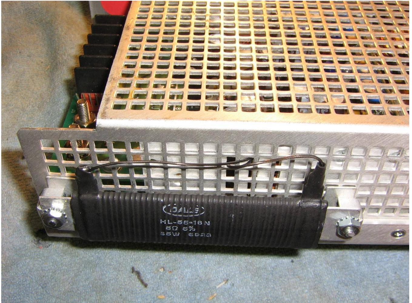
5 ohm / 55 watt load resistor across the +5 VDC output.
