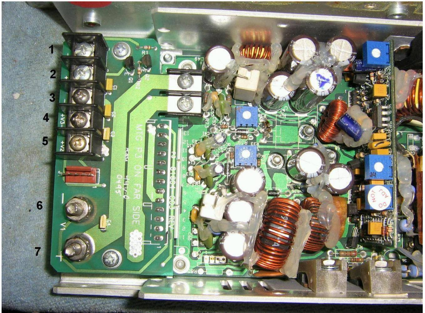
Closeup view of the Xentek's power supply's output terminals.
