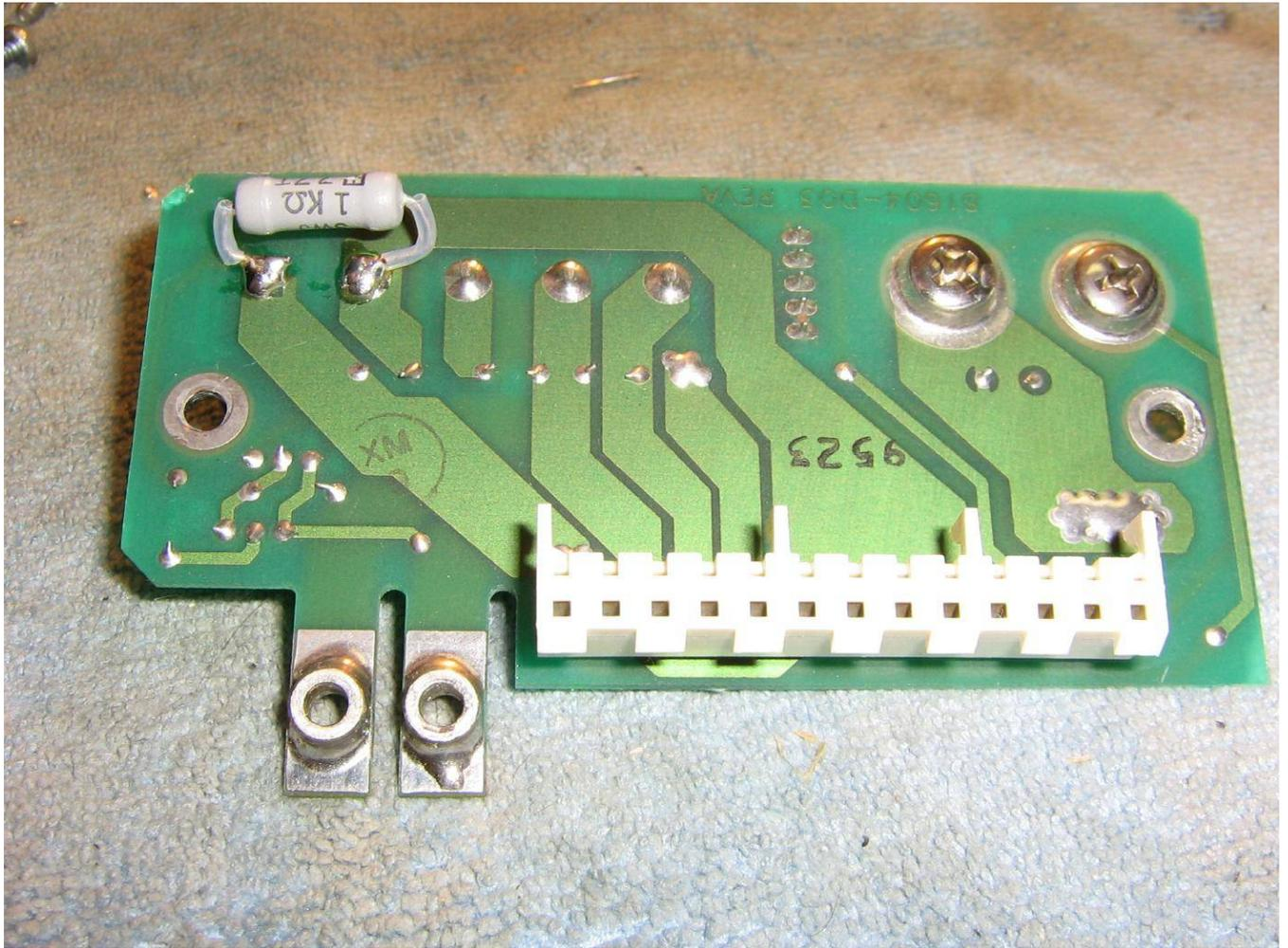
1k ohm / 3 watt load resistor across the +24 VDC output.
