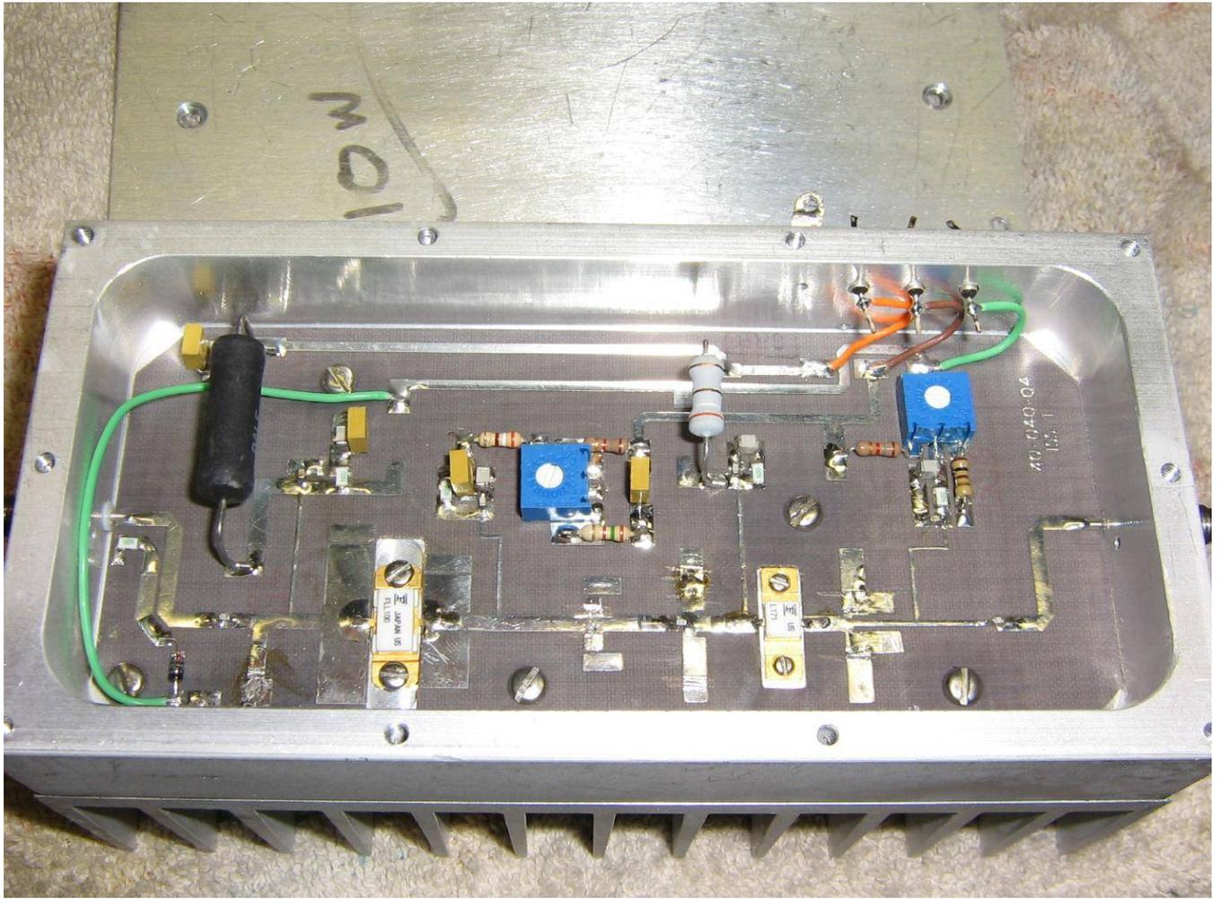
Internal view of the Comwave 10 watt MMDS amplifier.
