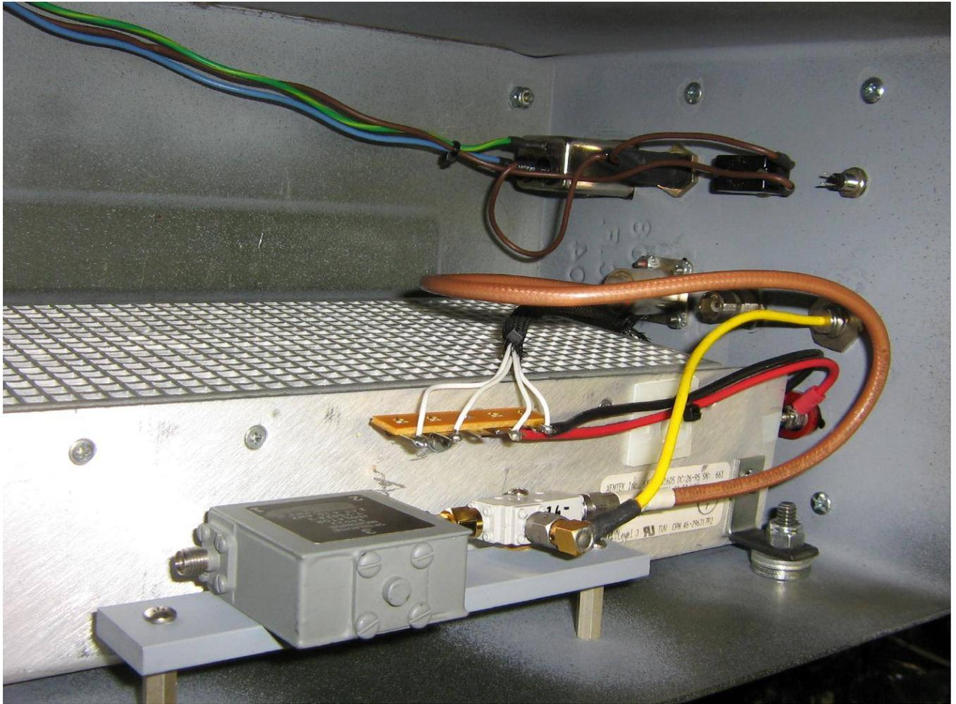
Mounting the ferrite isolator and directional coupler.
