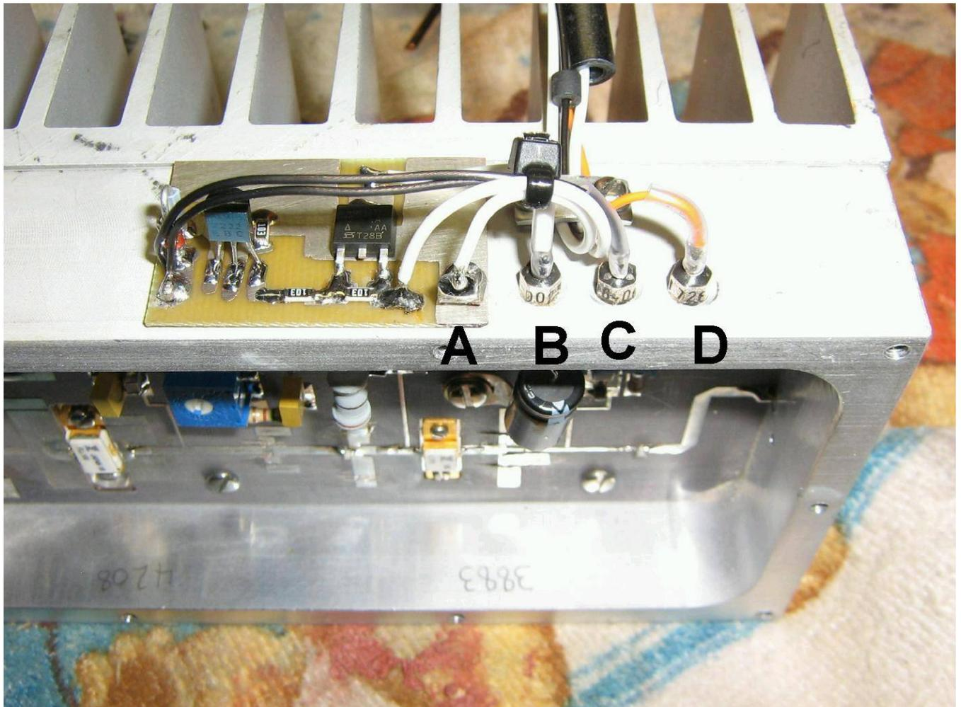
Closeup view of the negative voltage sequencer circuit board and the amplifier's DC power connections.
