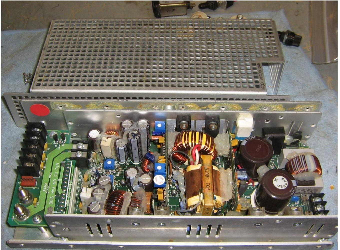
Internal view of the Xentek switching power supply, Fair Radio part number SX200-81605.
