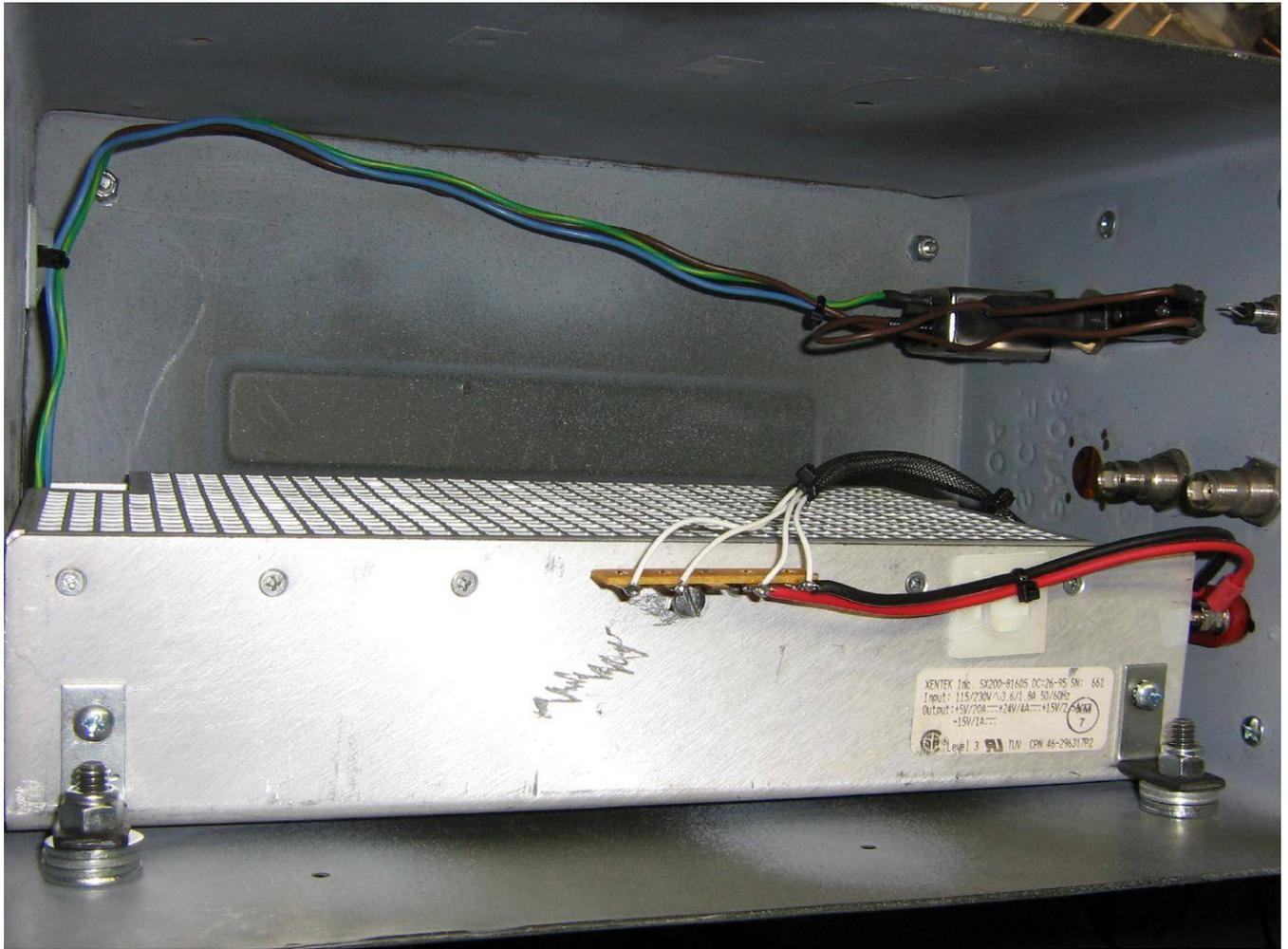
Mounting the switching power supply inside the project case.
