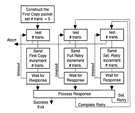
Figure 8-4 Confirmed Delivery Packet Transmission State Diagram
