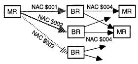
Figure 3-1 Separated Repeaters Servicing a Wide Area
