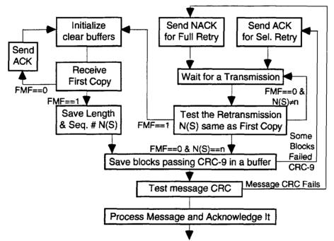
Figure 9-1 Confirmed Delivery Packet Reception State Diagram
