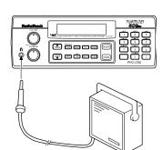
Note: Connecting an external speaker disconnects the scanner's internal speaker.
