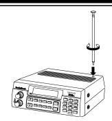
The scanner's sensitivity depends on the antenna's length and various environmental conditions. For the best reception of the transmissions you want to hear, adjust the antenna's length.
