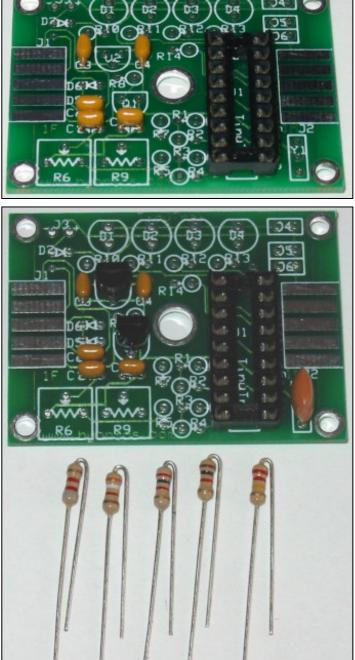
Install resistor R8. (2.2K, red-red). Use instructions for resistors above. Note: If TinyTrak3 will be used with a radio that does not key via current through the microphone line, such as mobile radios and Kenwood handhelds, R8 will not be needed. If R8 is used, you should not wire PTT OUT to the radio.
