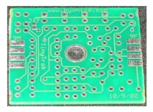
If TinyTrak3 is ordered without a case, the PCB will have four mounting holes in the corners, as shown below.
