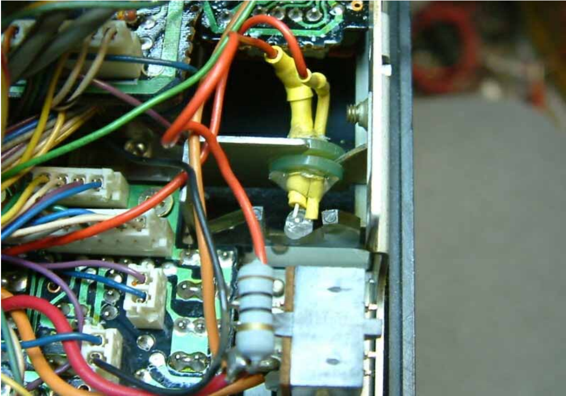
Picture 9: Completed LED assembly in it's new home! Tuck the wires so that they don't get pinched when you put the CW/VOX switch or the display unit back in place.
