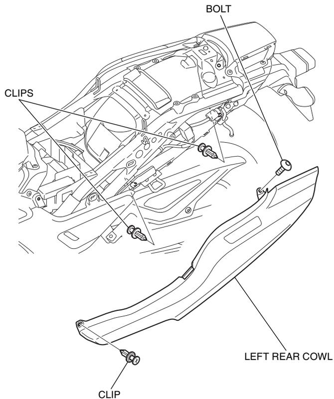
3. Refer to the Service Manual for the motorcycle, remove the covers from the inside of the rear cowls.
