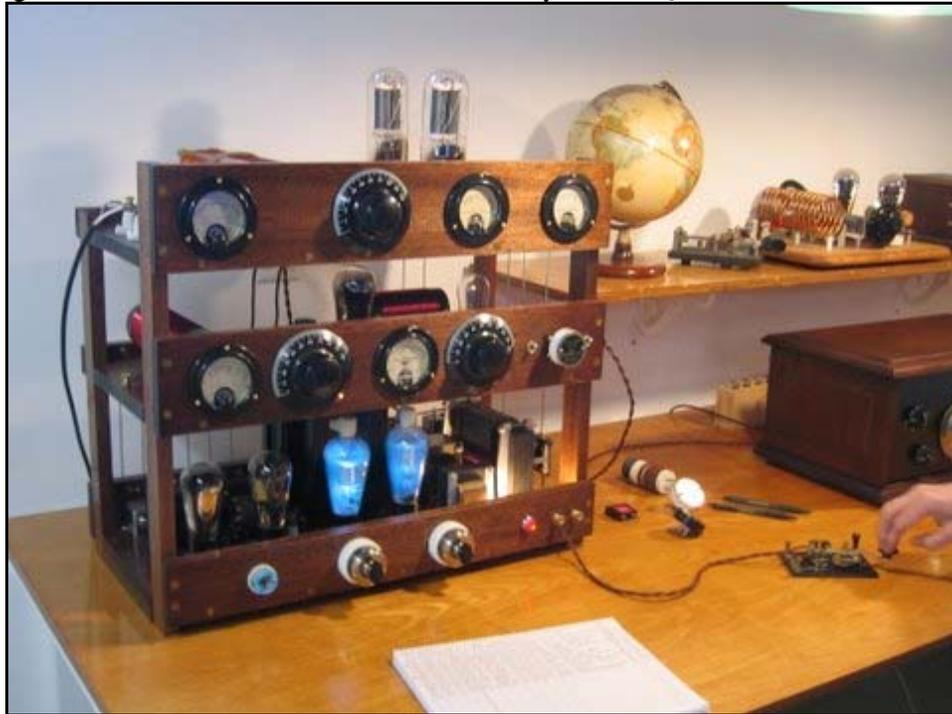
The transmitter uses a combination of circuits from early ARRL Handbooks, and uses only parts that were available by 1929. A pair of "50 watters" are used to put out around 150 watts on 160 meters.
