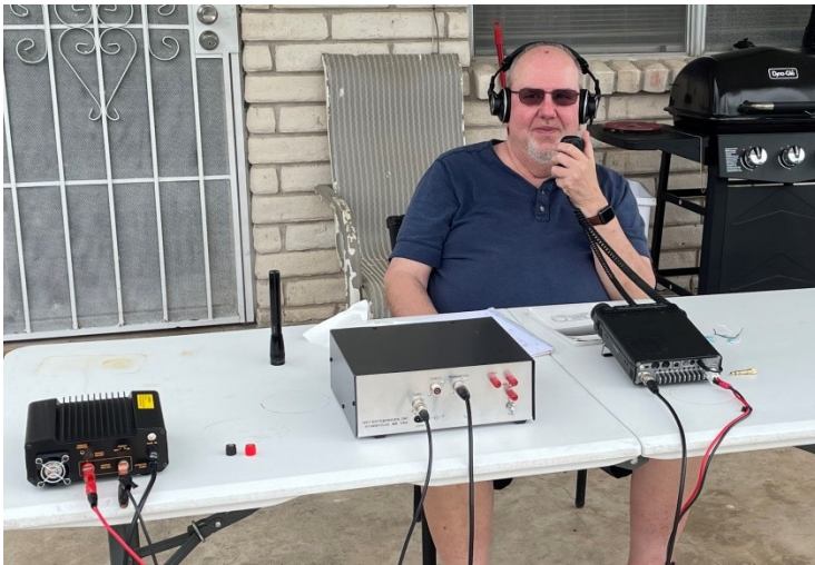
N8NAV/W5 operating from the back patio of our rented house in Brownsville, Texas. The rig is a Yaesu FT-891 with an MFJ-969 tuner and Alinco power supply.
